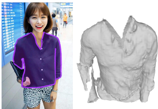
Figure 6: Example of poor reconstruction due to symmetry effects (back is assumed to be of same geometry as front).
